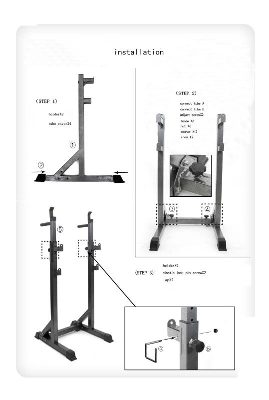
elastic lock pin screw out and pull back, can adjust the height
