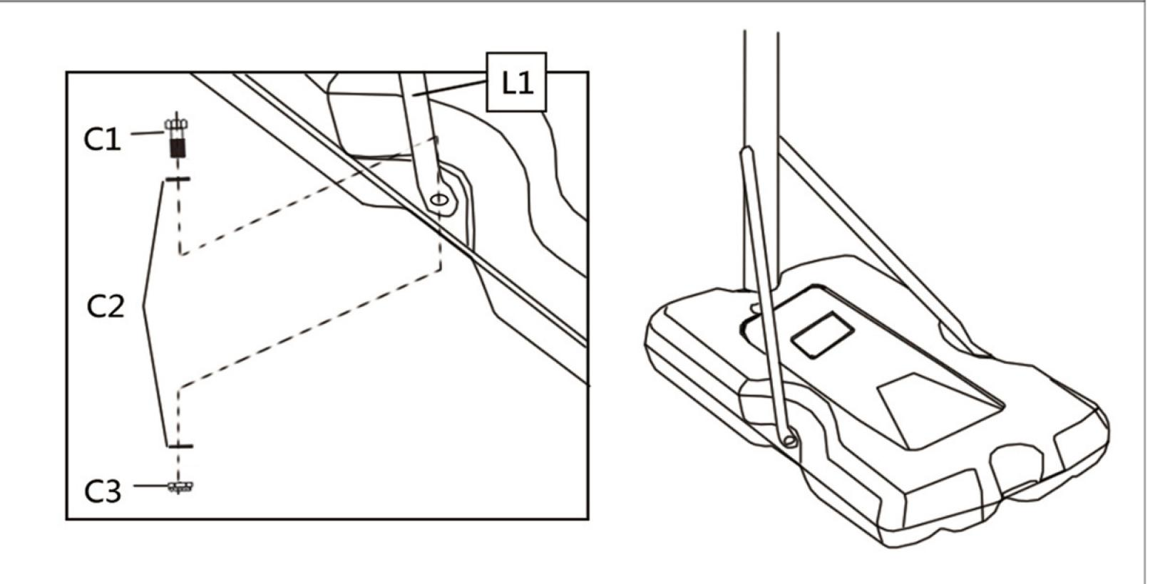
Fix the other end of Pole Brace(L1)&(L2) on two sides of Base(S) by Bolt Set (C1), (C2)&(C3) as shown.
