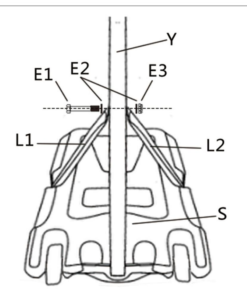
Fix one end of Pole Brace(L1)&(L2) on Bottom Pole(Y) by Bolt Set (E1),(E2)&(E3) as shown.
