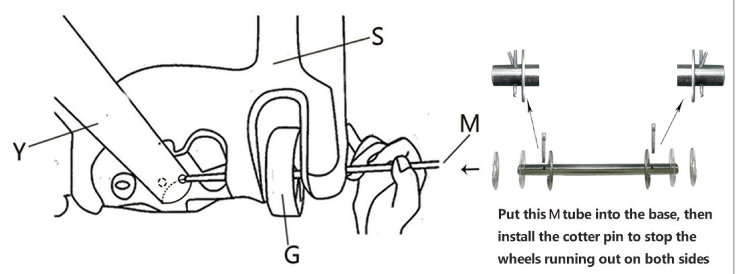
Insert the Wheel Shaft (M) into Wheel(G), Base(S) and end of Bottom Pole (Y) as shown.
